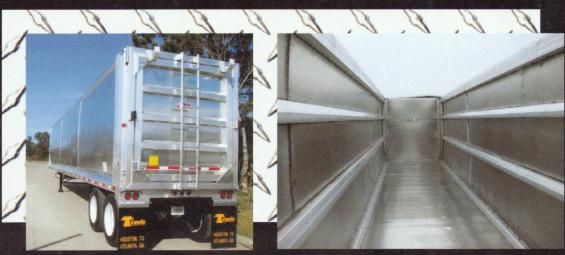
The slightly curved outer wall and formed outside shedder plate add strength and needed flexibility. Also shown is an optional air flow gate. Large inside horizontal beams replace the need for outside side stakes. The trailer cleans out well and is easy to repair when damaged.
